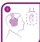
The ear cups should fit snugly against the head. To ensure an effective noise seal, adjust the ear cups and headband to the correct position on the head. Put the Ear Defenders on before exposure to noise. (Fig.3).
